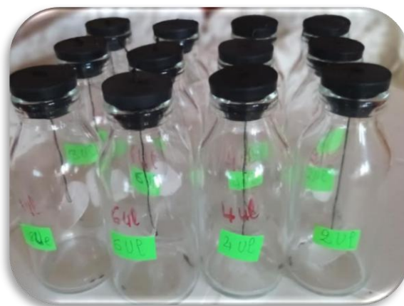
Fig. 4 : Experimental device of the test applied by inhalation with the essential oil of lemon C. limon on adults of T. castaneum (Originel, 2023).
