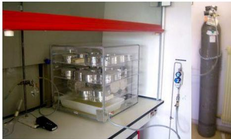
Fig. 3 : General view of the CRMD accelerated carbonation unit [1]
