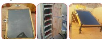
Fig. 1: Indirect solar dryer with forced and natural convection
