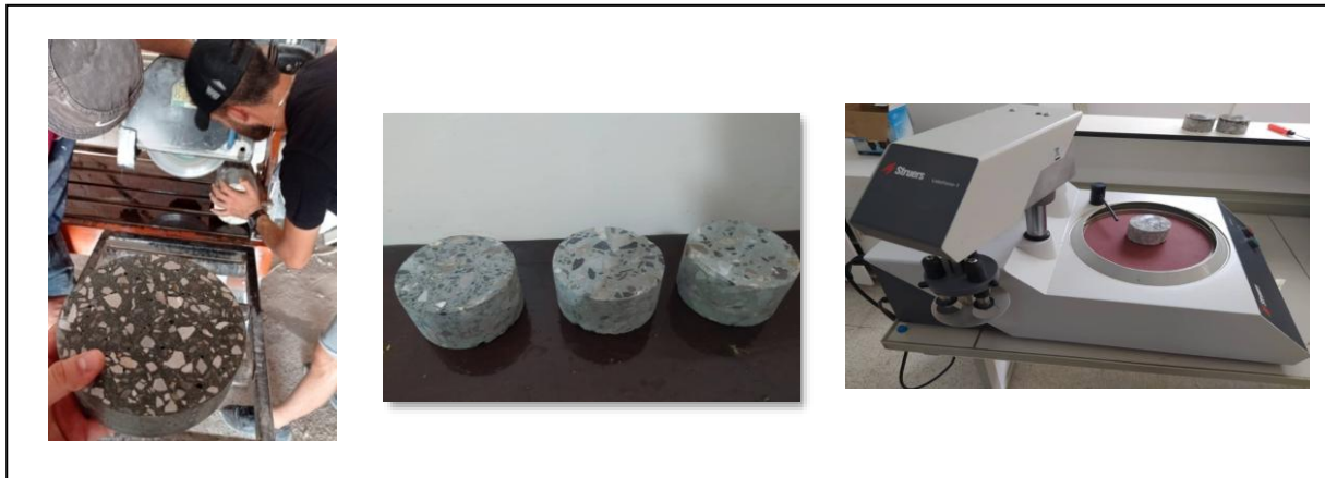
Fig.III. 1 : Cutting of the specimens with lapping and polishing.
