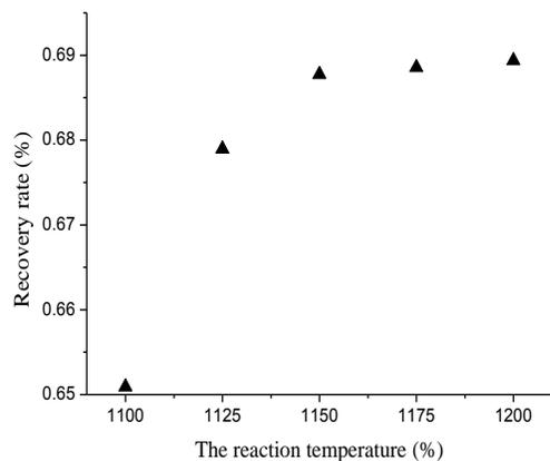
Fig. 4: The relationship between reaction temperature and the recovery rate of PbS.
