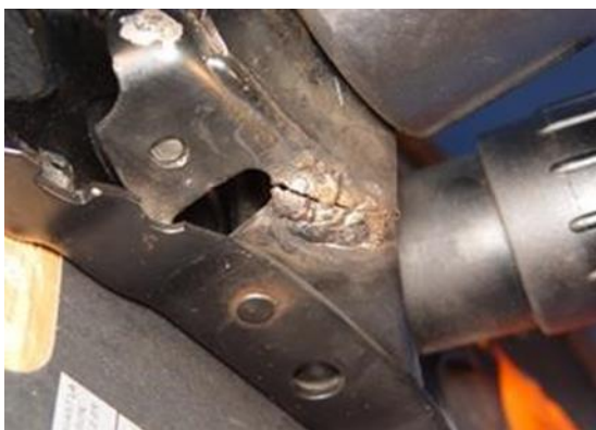
Fig.2 Failure due to residual stress
