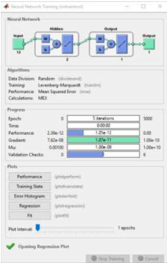
Fig. 2: summary of the results of backpropagation algorithm processing with Levenberg-Marquardt training method
